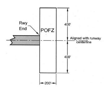
The POFZ is an 800 foot wide by 200 foot long area centered on the runway centerline adjacent to the runway threshold. The POFZ is only active when the ceiling (cloud layer) is less than 250 feet above the ground or the visibility is less than three-quarter (¾) statute miles. In addition, the POFZ is only active when an aircraft is on approach within two (2) miles of the runway.
